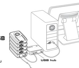
If your RocketPod stack is first in the chain (starting from the computer): As shown in the illustration at right, connect the DockPod to your computer; then connect the right-hand FireWire port of a stacked-on RocketPod module to the next FireWire device in the chain.
